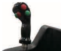
Forward/reverse and vibrating all controlled by the integrated control lever. The engine start is with neutral safety structure realised by the handle
