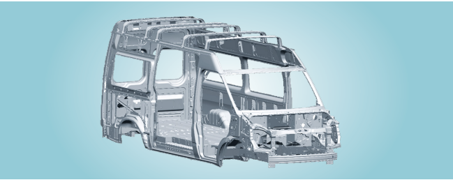
High-Strength Steel Coverage of 32% in Body Construction for Durability
