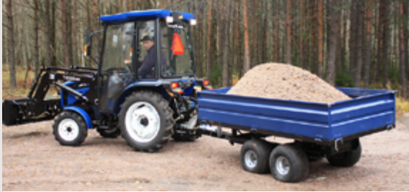
According to the height of the trailer, the hitch joint can be adjusted upwards or downwards to avoid hindering the output of PTO, which is convenient for users.
