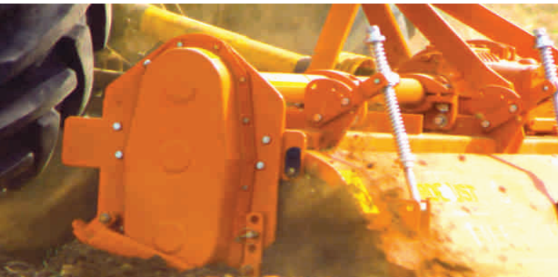
PTO shaft with overload protection
